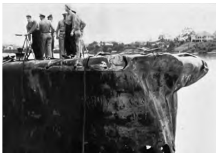
Navy personnel atop the Growler at Brisbane, Australia. The damage to a 25-foot section of the submarine's bow, which occurred when it was rammed by the 900-ton Japanese cargo ship Hayasaki , can be clearly seen.
